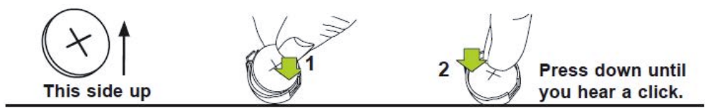
Figure 19. Install the battery
